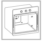
1. Loosen the two screws A (*see diagram*). If the oven is fitted with self-cleaning panels, these will have to be temporarily disassembled.
